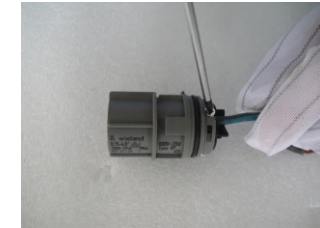
Figure 4.16 Connect Wires to the Terminal
