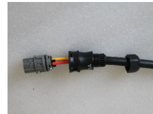
Figure 4.16 Connect Wires to the Terminal
